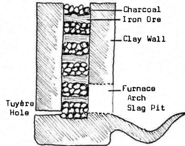
was reached the melted slag trickled out from the opening at the base of the shaft. The iron, a sponge-like mass, was left in the shaft. This had to be removed and reheated in an open bowl furnace and then hammered on an anvil. Only then did it become real iron which would be made or forged into an implement.
