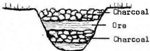
Evidence of smelting in the Bronze Age usually comprises a shallow clay lined bowl furnace with tiny remains of metal and slag, the melted rock waste, and charcoal.
