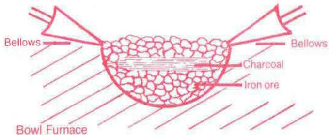
attached to a funnel. The use of such a funnel stops any back draught of hot gases into the bellows, a condition known as the 'Venturi effect'.
